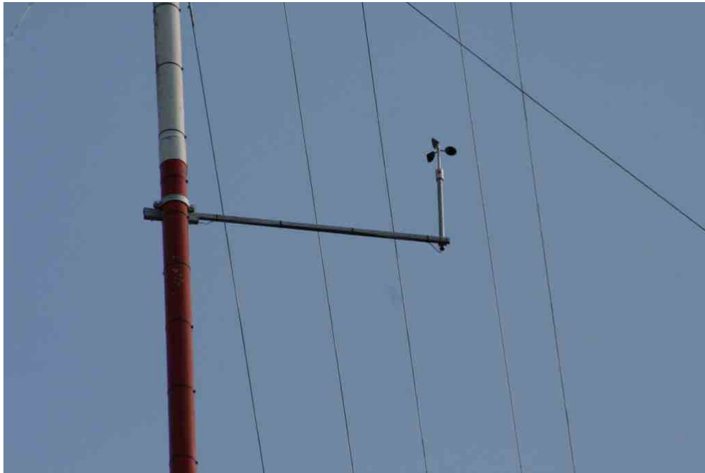
Figure 12: Installation of Wind Speed Sensor V4 (39,90m).
