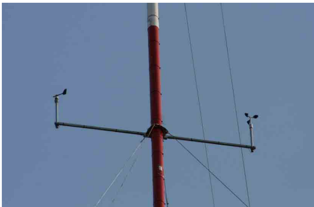
Figure 10: Installation of Wind Speed Sensor V3 (61,30m) and Wind Direction Sensor D2 (61,20m).
