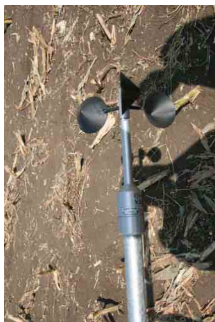
Figure 10: Installation of Wind Speed Sensor V3 (61,30m) and Wind Direction Sensor D2 (61,20m).
