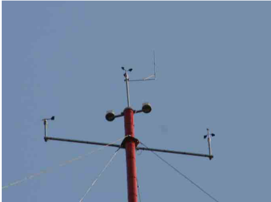
Figure 6: Installation of Wind Speed Sensor V1 (85,80m), V2 (83,70m), Aviation light (83,80m) and Wind Direction Sensor D1 (83,60m).
