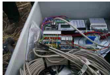
Figure 4: Instrument box with battery, data logger, charge regulator, barometric sensor and satellite modem.
