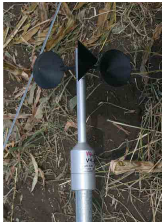
Figure 12: Installation of Wind Speed Sensor V4 (39,90m).
